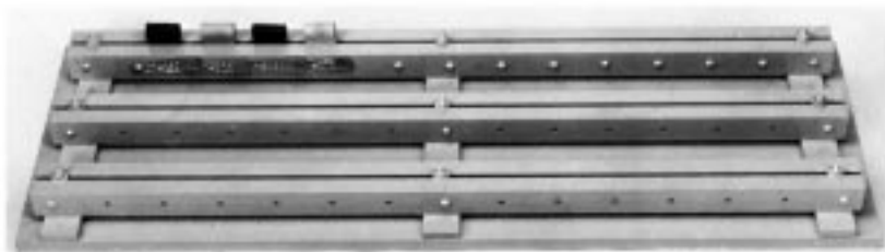
FIG. 3 Assembled Panel, Showing Method of Mounting Looped Specimens
