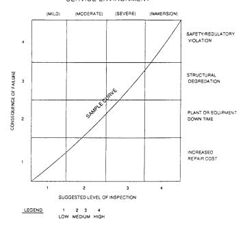
Note 1—This figure is provided as a visual aid to represent graphically the general relationship between the consequence of failure and the suggested level of inspection. The slope and configuration of the curve will vary due to the many factors affecting the consequence of failure, however, the suggested level of inspection should increase when the service environment is more severe.
