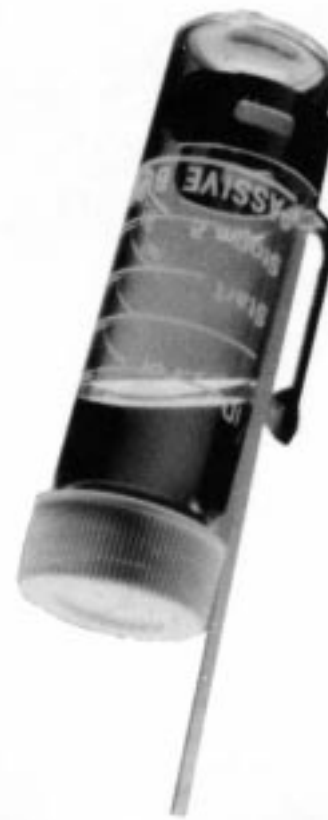
FIG. 1 Passive Sampler Showing Vial, Septum Cap Retaining Knudsen Disk, and Clip for Affixing Sampler for Personal or Area Samples
