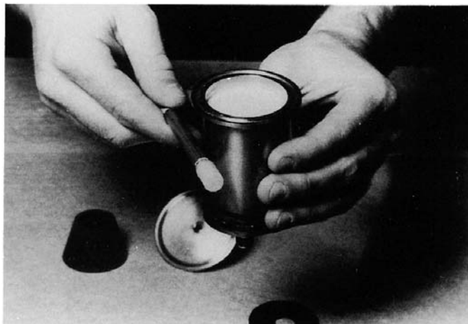
NOTE—Insert cone spacer, (large end of cone on top). Pour clay into cavity. Repeatedly, tap holder and add clay until level with top of cone. FIG. 4 Clay Cone Spacer
