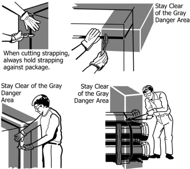
FIG. 2 Strap Cutting Techniques
