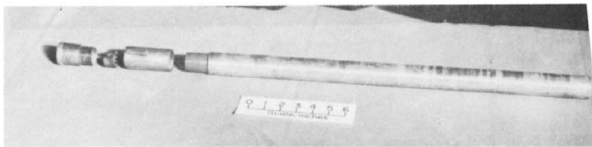
FIG. A1.1 EX Size Bit with Core Spring, Reamer, and 2-ft (0.7 m) EWX Core Barrel
