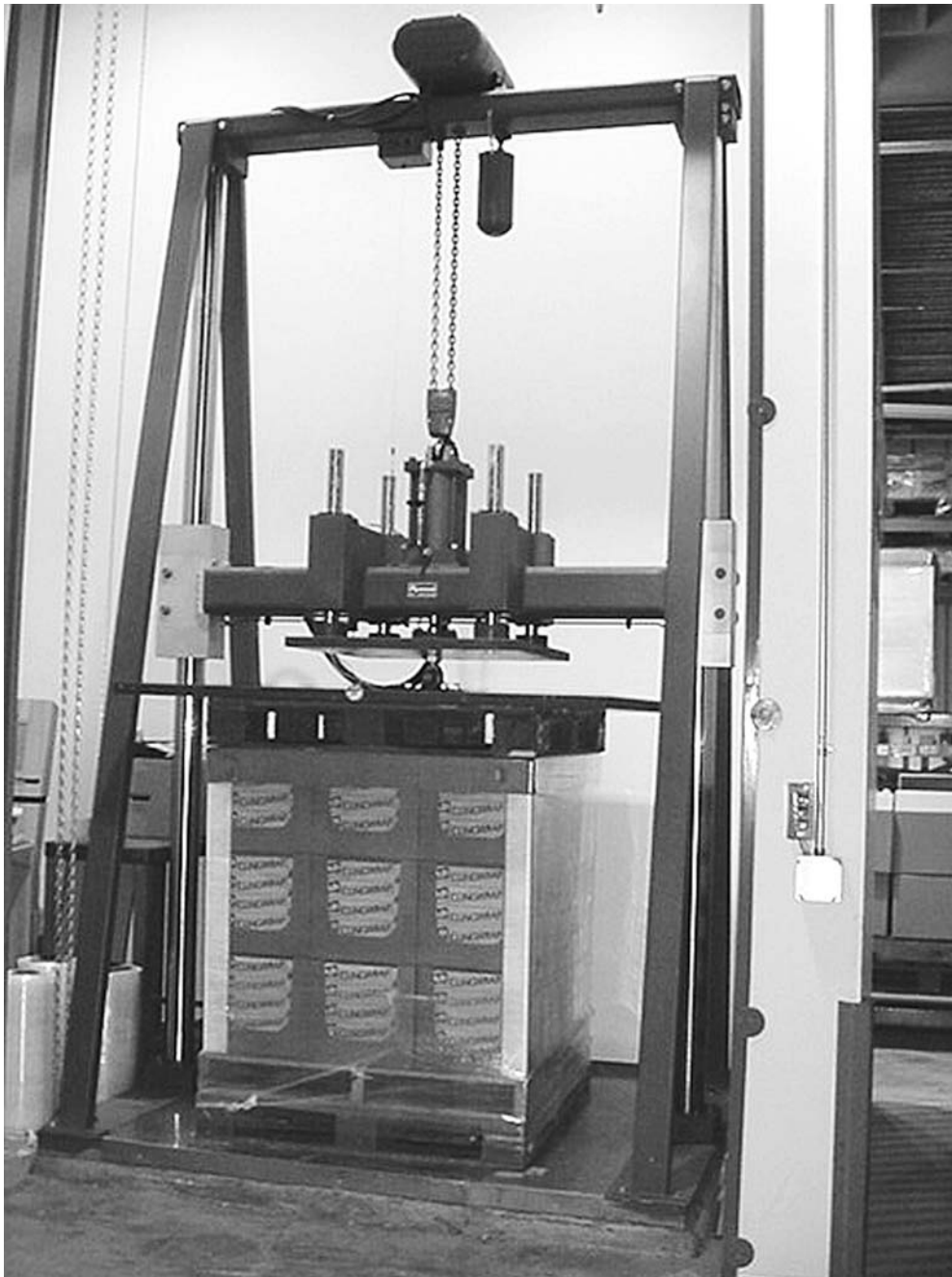
FIG. 4 Unitized Load Under Constant Load in Compression Machine With Swivel (Floating) Platen
