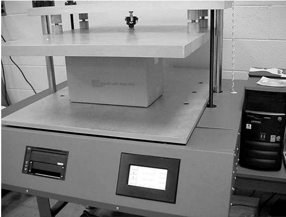
FIG. 3 Container Under Constant Load in Compression Test Machine With Fixed Platen
