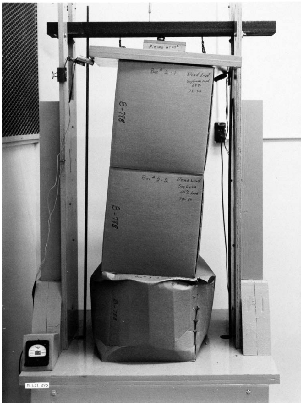
FIG. 1 Containers Under Constant Load of Dead Weights Imposed by Other Containers
