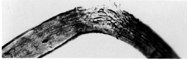
SEMI-RUPTURE AND DEVELOPING SPLIT
