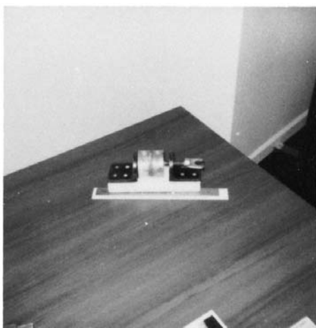
FIG. 1 Cell For Volume Resistivity 1-in. 2 Electrode (Mercury)
