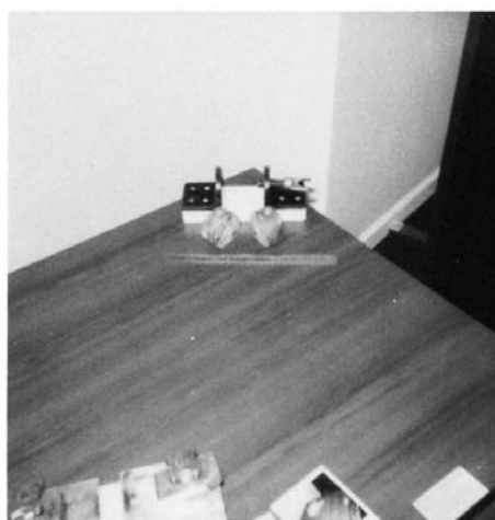
FIG. 1 Cell For Volume Resistivity 1-in. 2 Electrode (Mercury)
