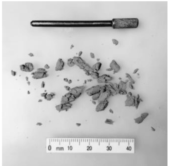
FIG. X2.4 Example of Soil at the Plastic Limit
