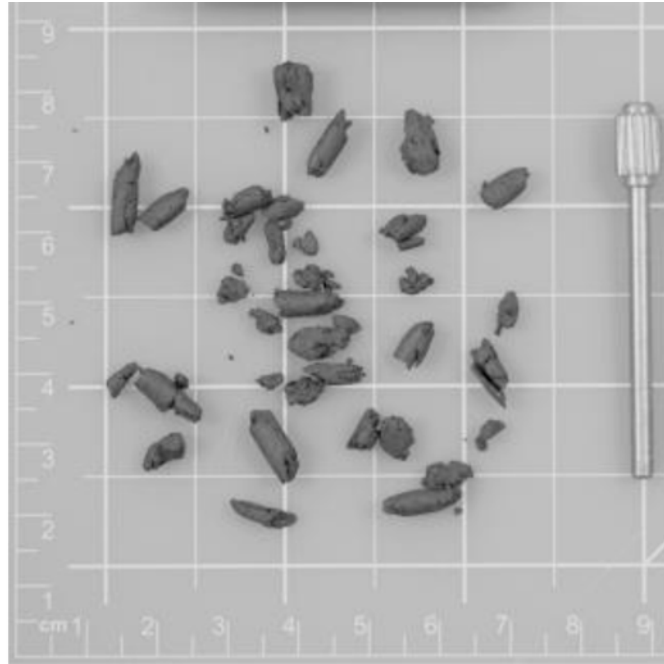
FIG. X2.7 Example of Soil at the Plastic Limit
