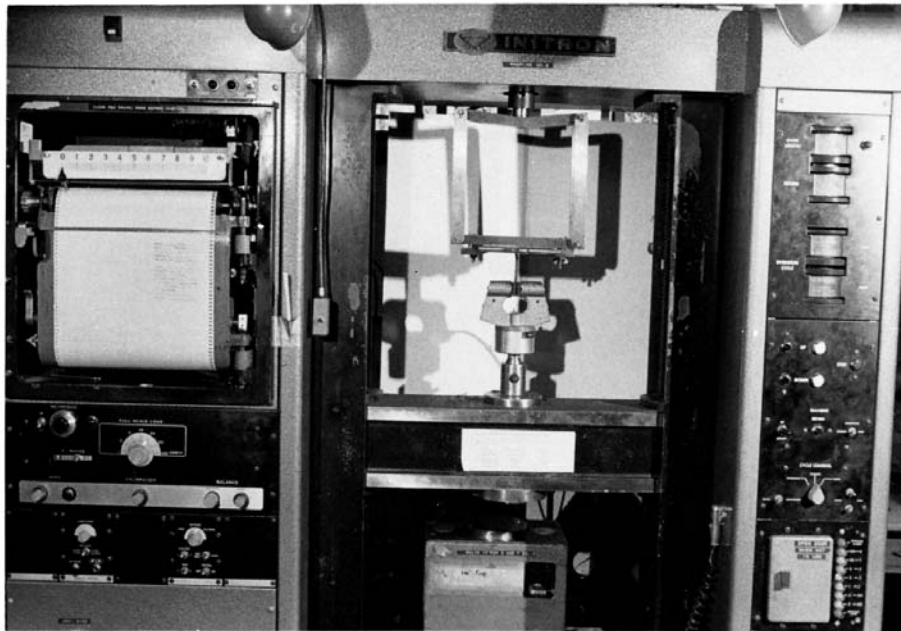
FIG. 14 An Example of a Rubber Tank Lining Adhesion Specimen in a Testing Machine
