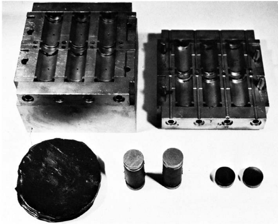
FIG. 8 Mold and Conical Test Specimens
