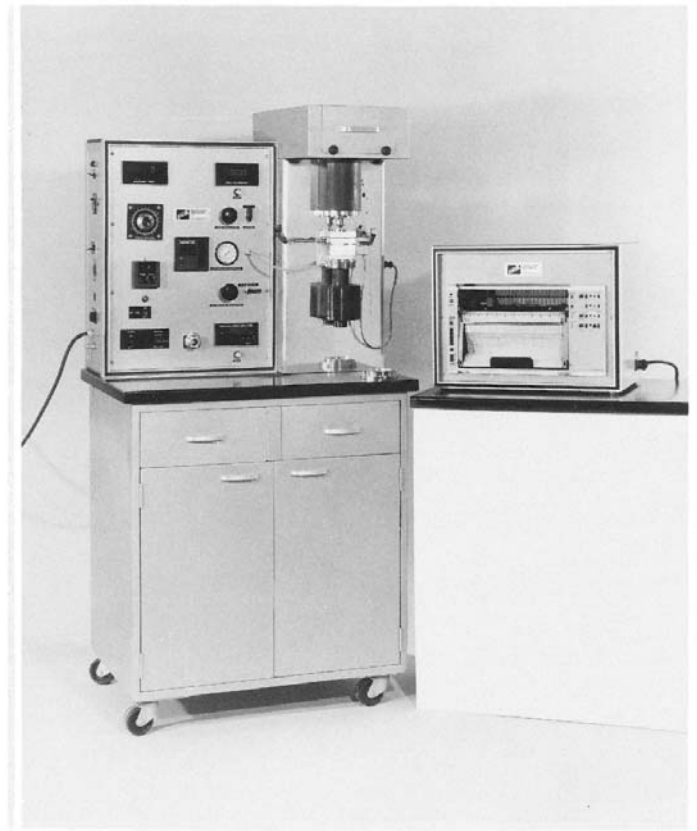
FIG. 3 Falex Variable-Speed Four-Ball Wear Test Machine
