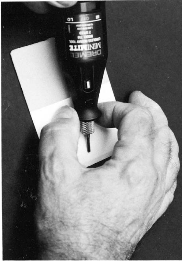
FIG. 4 Holding Rotary Tool for Grinding
