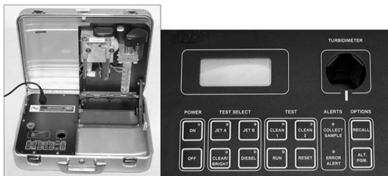
FIG. 2 Micro-Separometer Mark X and Associated Control Panel
