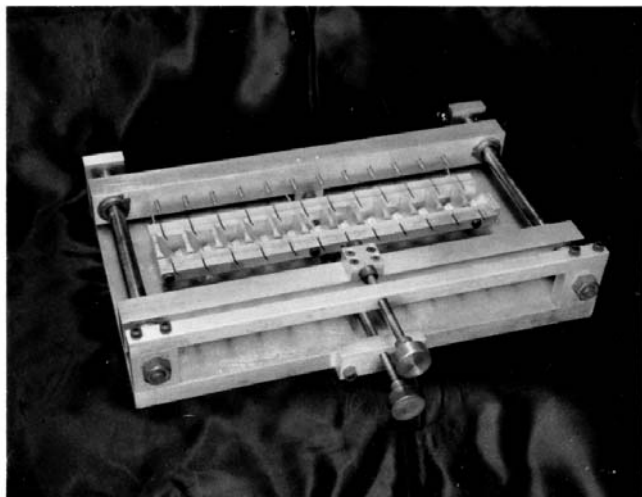
FIG. 3 Needle Insertion Jig
