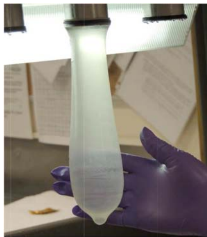
FIG. A3.2 Leakage Test
