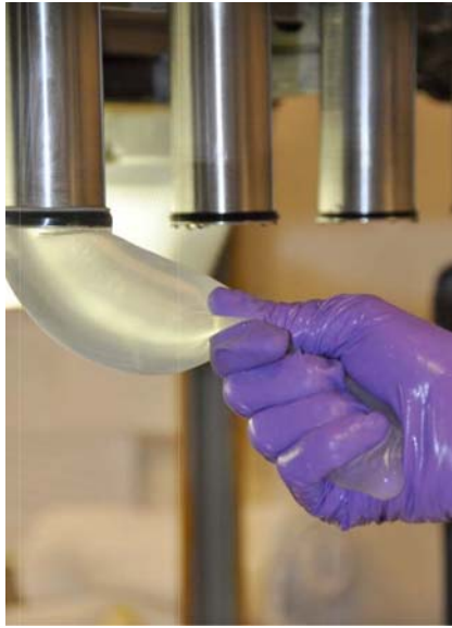
FIG. A3.3 Leakage Test
