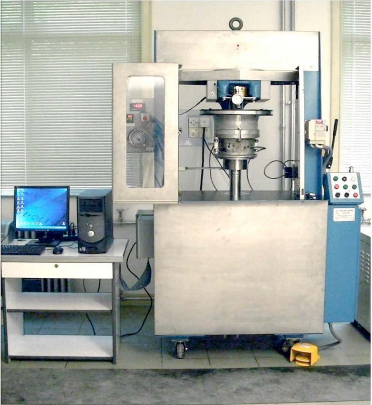
FIG. 2 GTM Compaction and Shear Test
