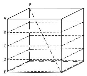
Note 1—A is the top surface immediately upon exposure; B is the surface exposed on removal of the first quarter, C is the surface at the middle of the bale; D is the surface exposed on removal of three fourths of the fiber, and E is the surface 2 to 3 cm above the bottom of the bale, F is the diagonal through the center of the bale.
