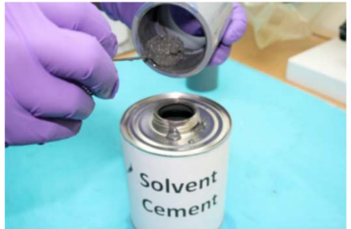
FIG. 14 Apply a thin and even layer of solvent cement inside the socket.
