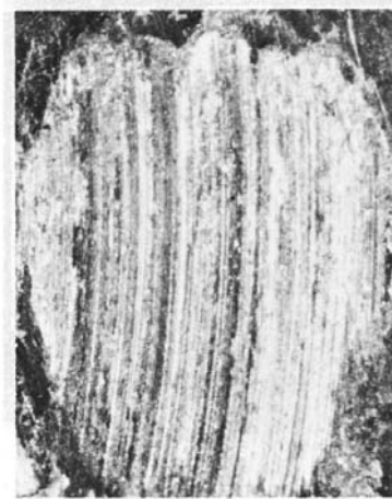
FIG. 7 Typical Test Ball Scars—After Removal
