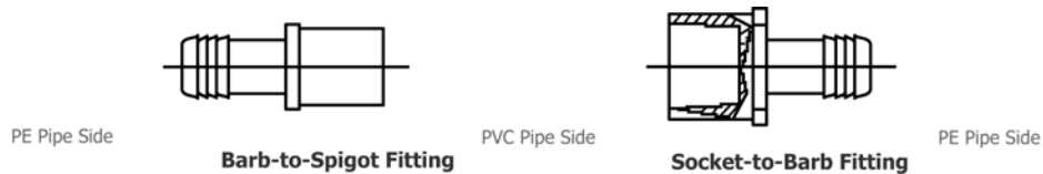
FIG. 1 Illustration of Typical PE-to-PVC Transition Fittings.
