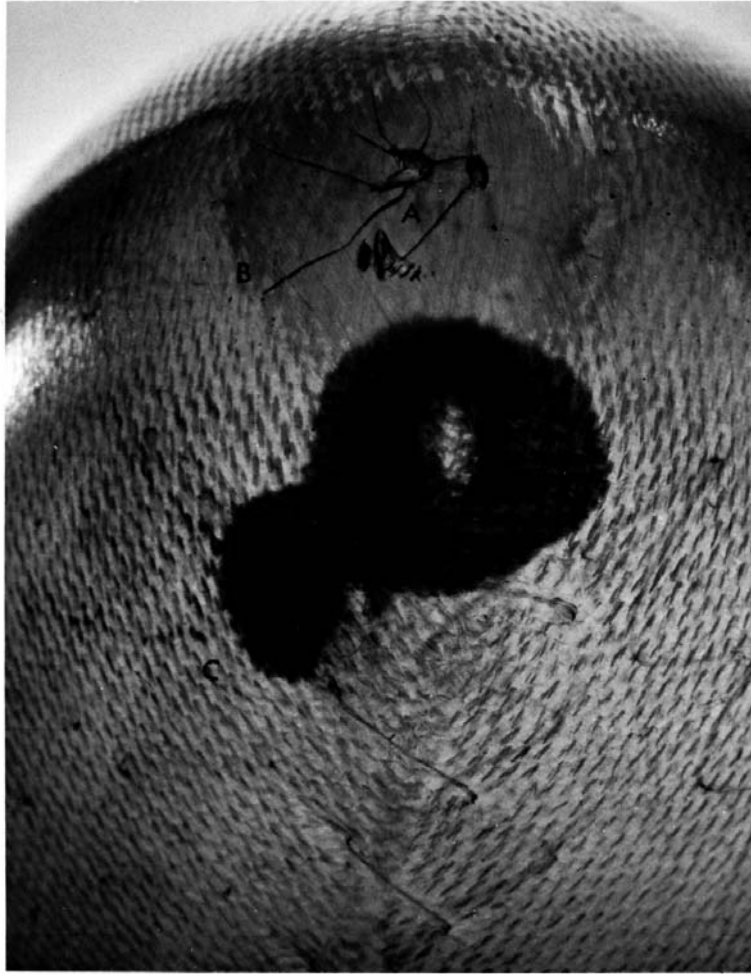
FIG. 1 Chips (A), Surface Cracks (B), Interply Delamination (C)
