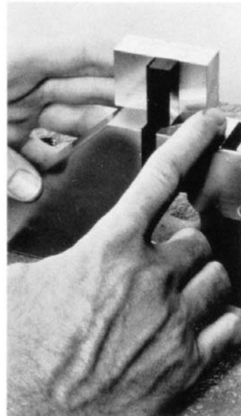
FIG. 4 Jig for Positioning Specimen for Clamping
