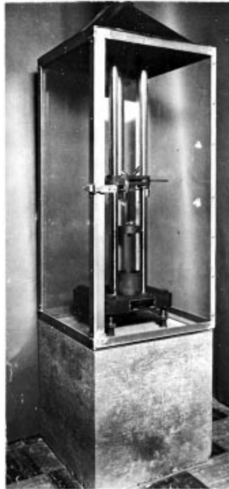
FIG. 7 Drop-Weight Tester in a Protective Enclosure
