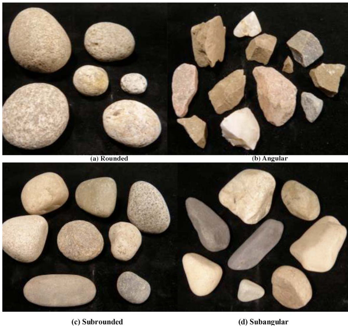
FIG. 3 Typical Angularity of Bulky Grains
