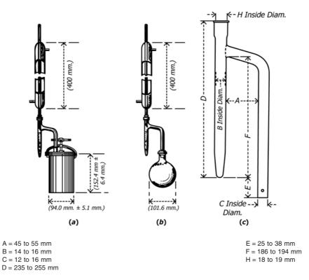
FIG. 1 Apparatus for Determining Water Content
