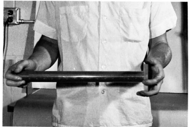
FIG. 7 Using Hand Method of Shaking
