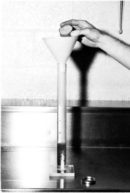
FIG. 5 Transfer of Samples from Measuring Tin to Cylinder
