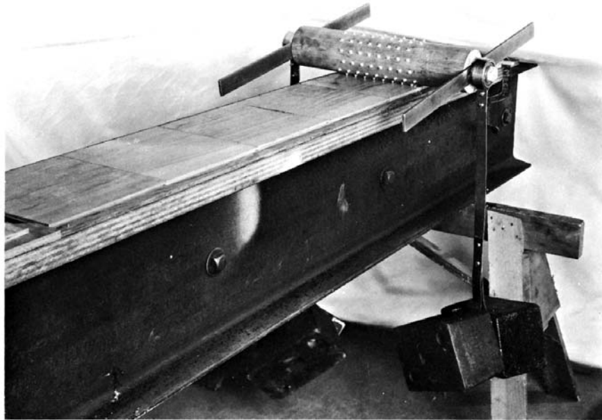
FIG. 3 Assembly for Tests of Floor-Surface Indentation from Small-Area Loads, Showing Loaded Maple Roller Studded with Boot Caulks and Specimens Firmly Supported on Heavy Beam
