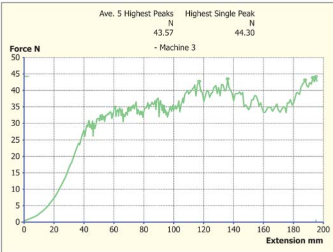
FIG. 4 Typical Tongue Tearing Force-Extension Curves for Individual Specimens (Typical woven woolen fabric)
