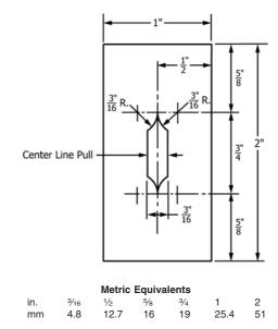
FIG. 2 Shape and Dimensions of Die for Cutting Slit Tear Test Specimens
