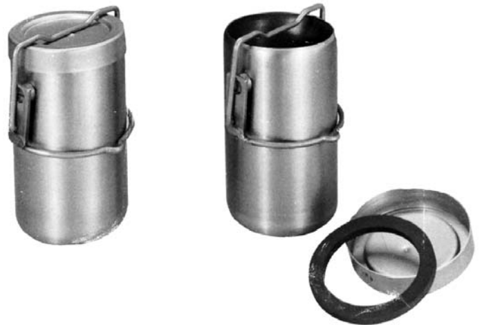
FIG. 4 Launder-Ometer Stainless Steel Specimen Containers (Procedure A)
