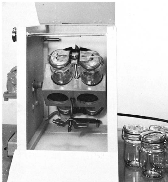
FIG. 1 Washing Machine, Heated Air Bath (Procedure B)
