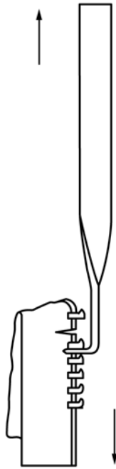
FIG. 2 Fixture for Element Slippage Test
