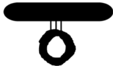
FIG. 5 Stab or Screw Shank Staple Buttons
