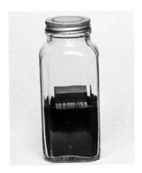
Note—In practice, the test block is not inserted until the bottle has been inoculated and the test fungus has covered the feeder strip. This figure illustrates the use of one feeder strip and one block. The use of larger bottles allowing two feeder strips and two blocks for each block is permitted (see 5.5).
