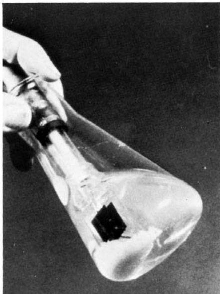
FIG. 2 Dip Cell Immersed in Flask
