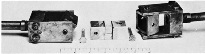
FIG. 4 Grip Assembly for Type B Specimen
