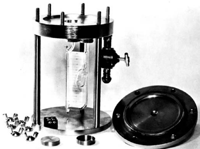
FIG. 1 Manometric Gas Transmission Cell
