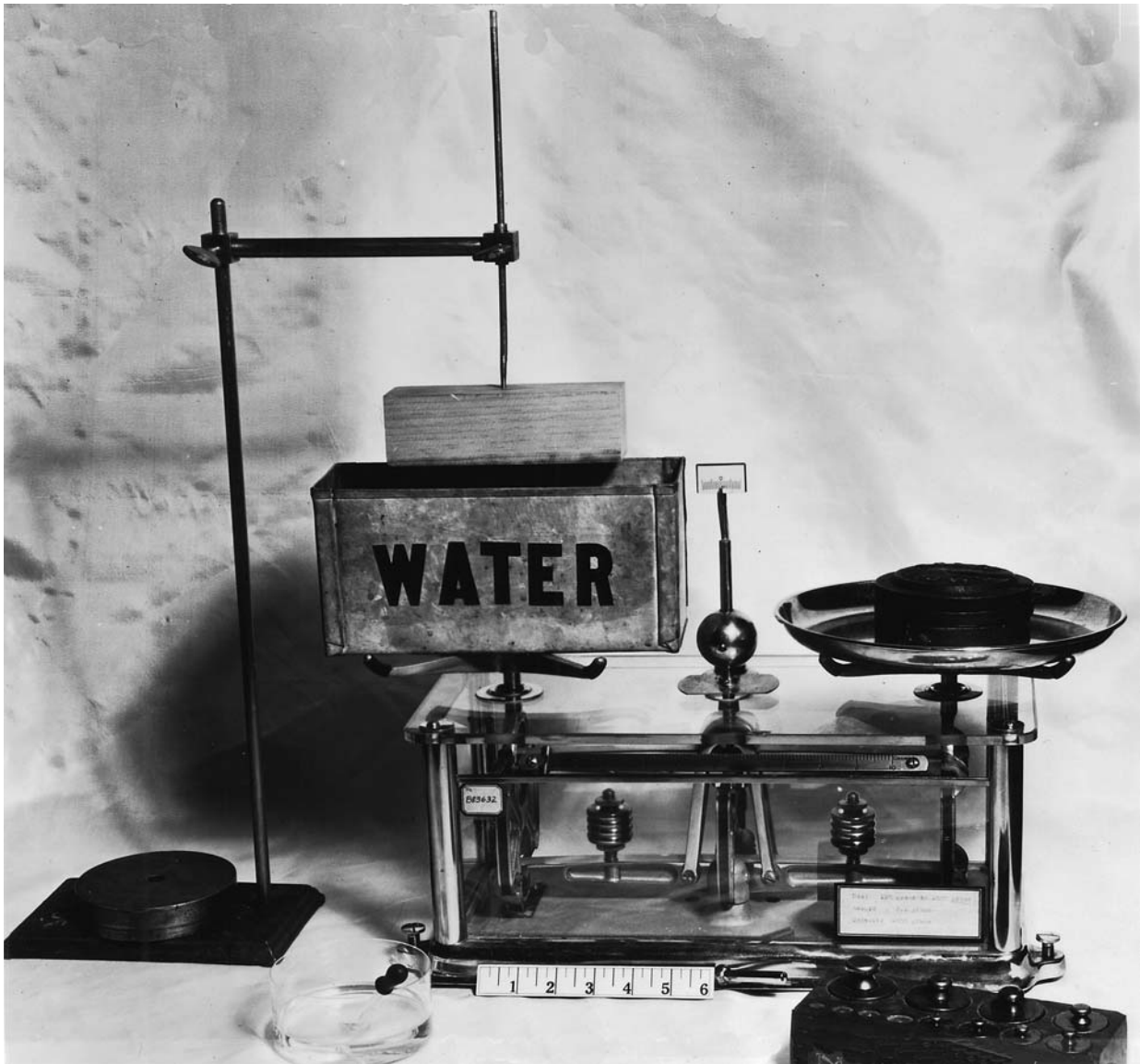
FIG. 40 Specific Gravity and Shrinkage-in-Volume Test Set-Up
