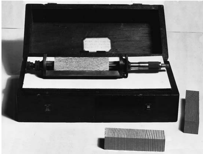
FIG. 42 Radial- and Tangential-Shrinkage Test Assembly
