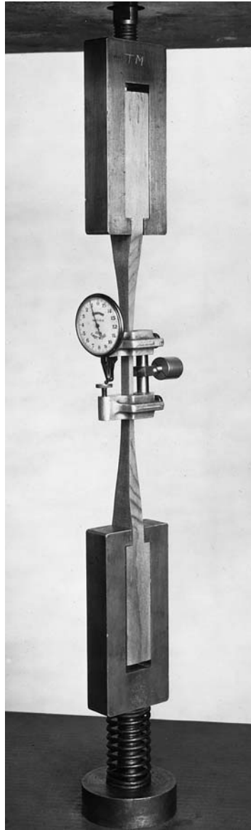
FIG. 30 Tension-Parallel-to-Grain Test Assembly Showing Grips and Use of 2 in. (50-mm) Gage Length Extensometer for Measuring Deformation
