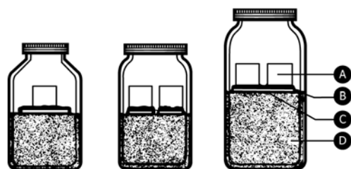
A—Wood cubes, 19-mm or 0.75-in. B—Test fungus growing over feeder block. C—Wood feeder strip, one feeder strip for each culture bottle.. D—Soil.
