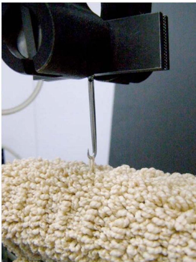
FIG. 4 Loop Hook Secured in the Upper Clamp (Note the hook has been passed through the loop)
