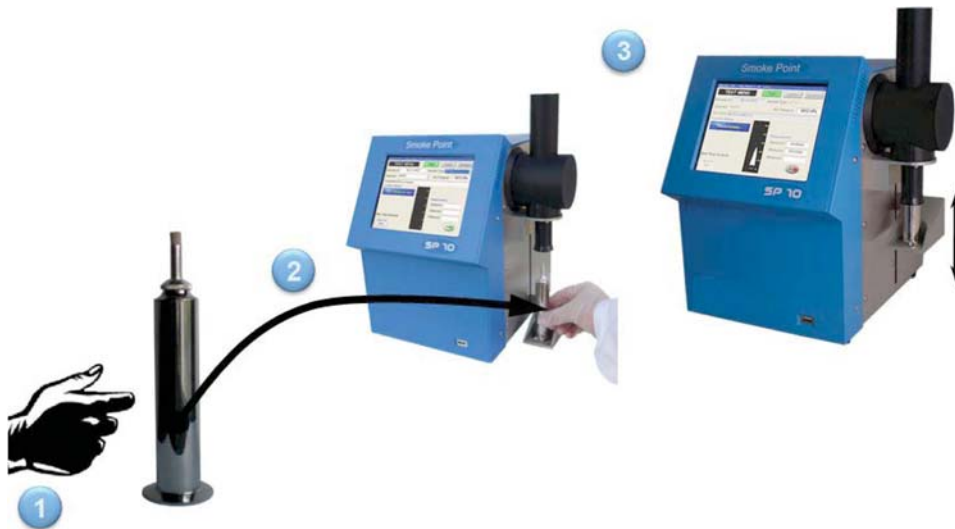
FIG. 8 Candle Positioning with Automated Apparatus
