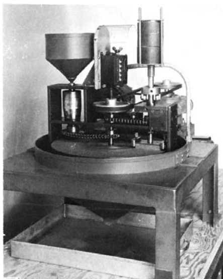
FIG. 23 Navy-Type Wear Machine for Abrasion Resistance Test
