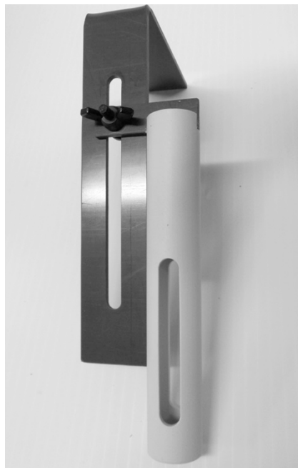
FIG. 3 In-site 1 Plating Device
