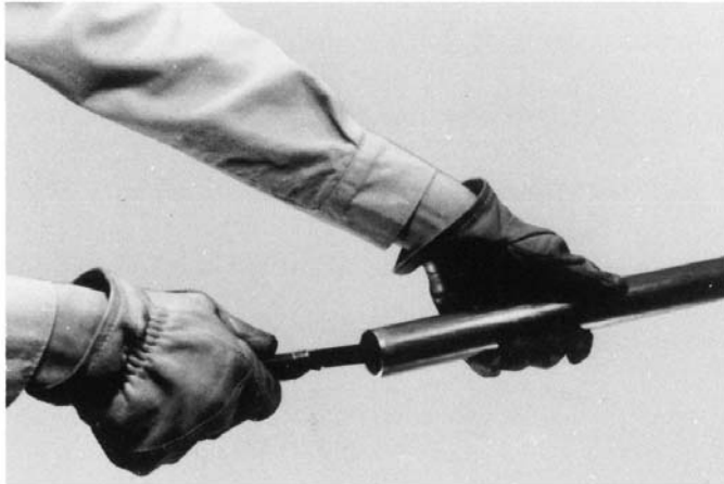
FIG. 4 Reaming: Pocket Knife
