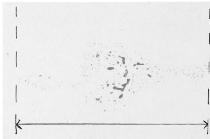
FIG. 4 Example of a spotty oxide inclusion. The maximum Feret's diameter is indicated.
