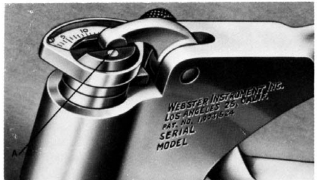
FIG. 3 Zero Adjustment Screw, A (indicated by arrow)
