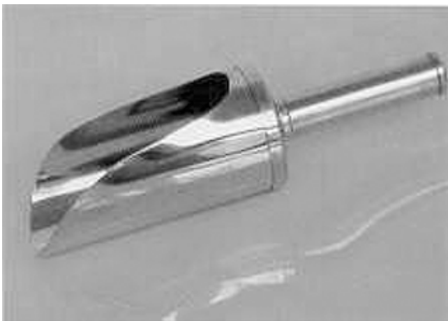
FIG. 4 Stainless Steel Scoop for Sampling Metal Powder
